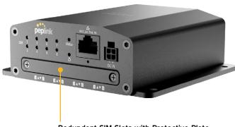
Redundant SIM Slots with Protective Plate
